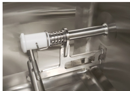
Active Coupler inside Wash Chamber
