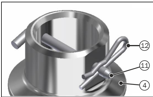
Picture 5.2-7: Clip-on connection
