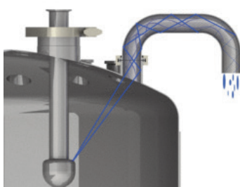
Tank Vent Solution Loss During CIP
