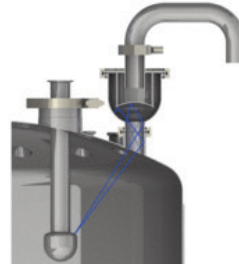
Hygienic Spray Deflector Preventing Solution Loss During CIP
